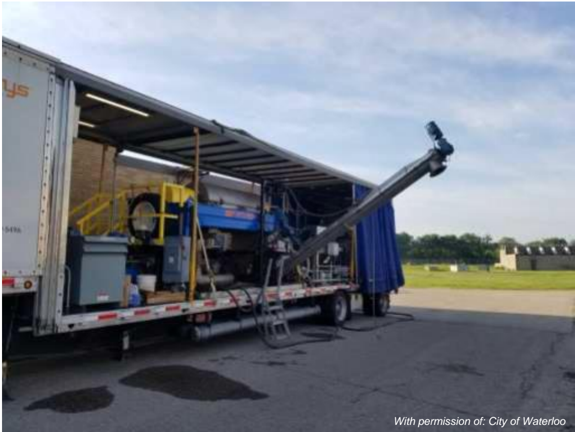
Centrisys dewatering centrifuge pilot test setup at the WWTP, June 2018
